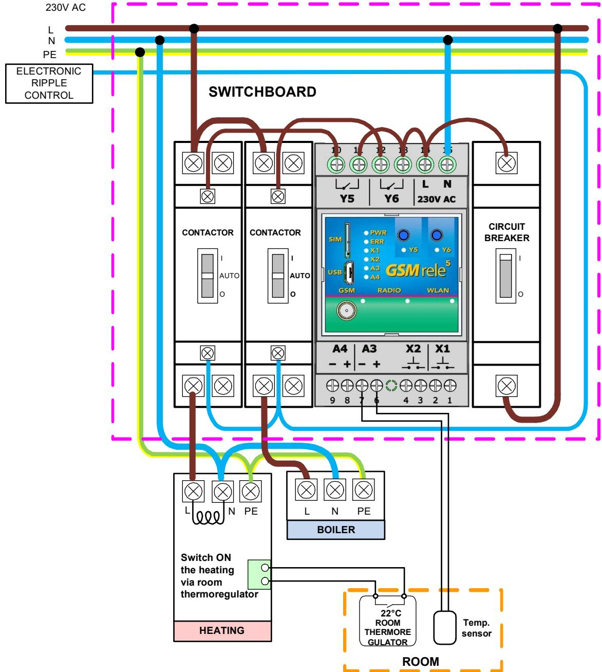
This wiring works like that. Temperature sensor A3 is able to regulate (switch on/off) output V3. Switching output V3 on/off by temperature sensor A3 is set in factory configuration.
