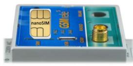
4. Now it's possible to connect the device to 230V AC power supply. If the power supply is correct, green LED **PWR** goes on and blue LED **GSM** is flashing slowly. After about 20 seconds, blue LED diode **GSM** starts flashing with a period 1 per 3 sec. (registered).
