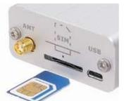
Above the SIM card holder is located the LED which indicates status of GSM.
