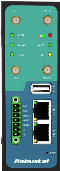
Each Ethernet port has two LED indicators (please check the following picture). The yellow one is **Speed indicator** and the green one is **Link indicator**. There are three status of each indicator. For details please refer to the form below.
