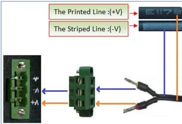
The power supply range is 9 to 60 VDC.
