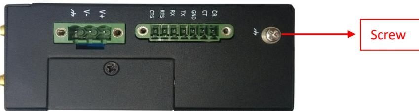
**Note:** This product is intended to be mounted to a well-grounded mounting surface, such as a metal panel.
