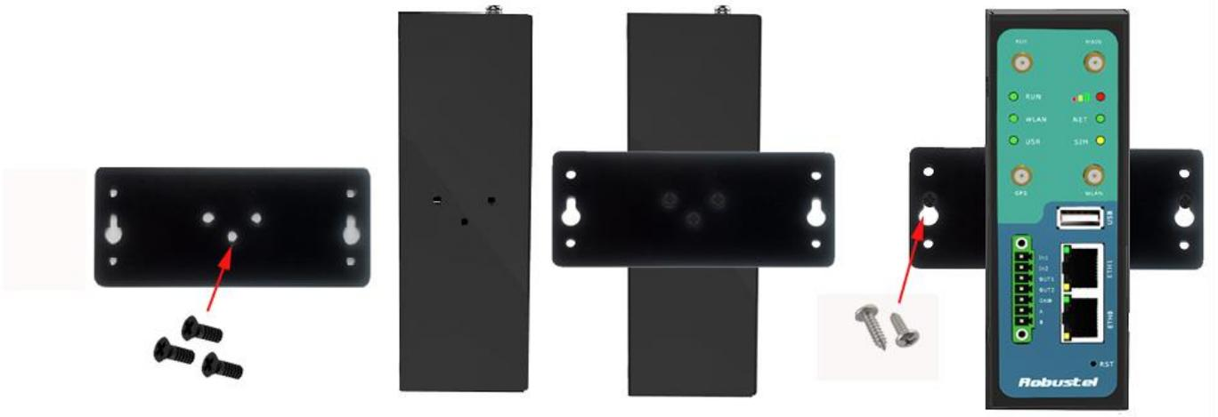
2. Mount the router on a DIN rail with 3 pcs of M3 screws, and then hang the DIN-Rail on the holder.
