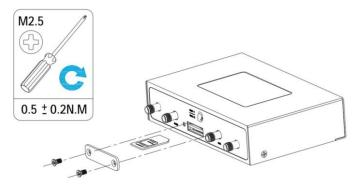
Insert or remove the SIM card as shown in the following steps.
