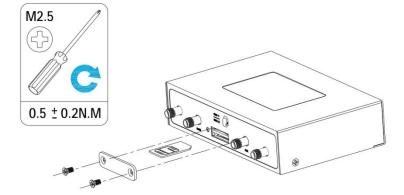
Insert or remove the SIM card as shown in the following steps.
