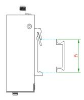
Use 3 pcs of M3\*6 flat head Phillips screws to fix the DIN rail to the router, and then hang the DIN rail on the mounting bracket. It is necessary to choose a standard bracket.
