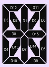
The D0~D15 of right most digit of alphanumerical display board is mapped to SEG0~SEG15 while the D0~D15 of the left most digit is mapped to SEG63~SEG48. One 7SG1 module can control 4 digits of 16-segment display.
