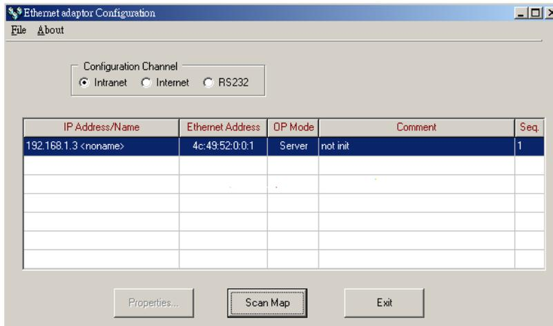
At that time, can double click the line where the desired Ethernet module is located or single click the line and click 'Properties..' button to perform the configuration. If password not setting or correct password were entered will show the screen as below
