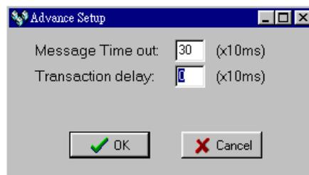
**Message Time Out** : The time-out time for PLC, the default setting is 300ms. Ethernet module will wait for the same amount time of this field before the PLC can reply the command message.
