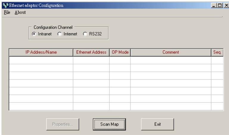
→ Click the 'Scan Map' button then start the scanning of Ethernet module. All the modules detected will be shown in the table.
