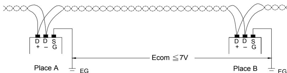
No matter how the ground potential is, we recommend using a twisted pair cable covered with shielding. The SG of each station is connected with the ground wire covered with shielding (similar to the above-mentioned "topology") to clear common mode voltage and provides the shortest circuit for signal transmission to improve the anti-noise capacity.
