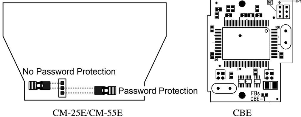
When CM-25E, CM-55E or CBE the jumper cap of JP1 is at upper position (linked by white line), the password protection is disabled. The jumper cap should put in the lower position when under normal operation.
