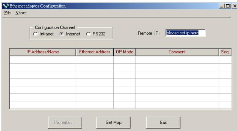
At this time can input the remote IP address of the Ethernet module desired for configuration. After click the 'Get Map' button, it will start to connect Ethernet module. When the connection is established will show the information regard the connected Ethernet module in the table at the middle of window.
