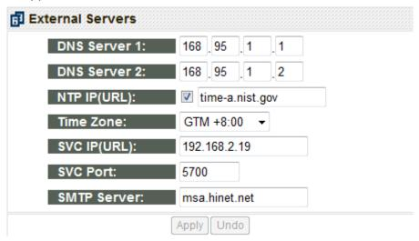
**DNS Server:** Domain name service server. Just like the primary DNS and secondary DNS set on the PC. This setting is not necessary if the network address setting is set to the dynamic (DHCP) mode. The preferred DNS setting in the figure below is the DNS server address of Chunghwa Telecommunications:
