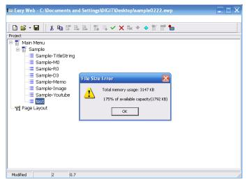
After confirming that the designed webpage content did not exceed the memory capacity provided by the FBs-CBEH series expansion board, click the OK button. Step 2, target IP and password input.
