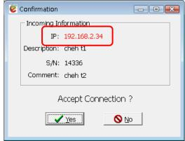
When the connection request window appears, the maintenance personnel can press the Yes button to accept this connection or press the No button to reject this connection.
