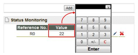
Here different pop-up windows will appear according to the data type and display formats; there are total of three types as shown below:
