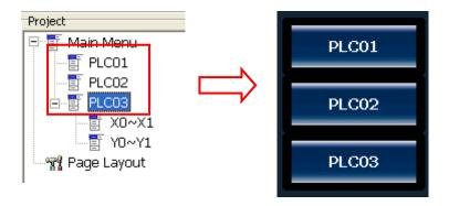
To add a second level sub-menu, just use the mouse and add a new menu in the first level menu just as described above, and as shown below, a sub-menu is added into the first level menu item.
