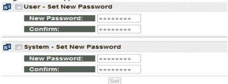
According to operation privilege differences, the CBEH module divides the password section into User password and System password. To enter an operation page, the user password or system password must be entered in order to log in; and to enter the system webpage, the system password must be entered to log in. There is no password set for the default factory user password, and the default factory system password is 1234.
