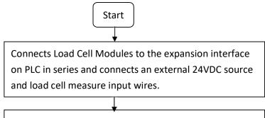
Execute the WinProladder and configure the load cell configuration table address, the register address, and working register in load cell configuration windows, then you can read the weight measurement value form register directly.
