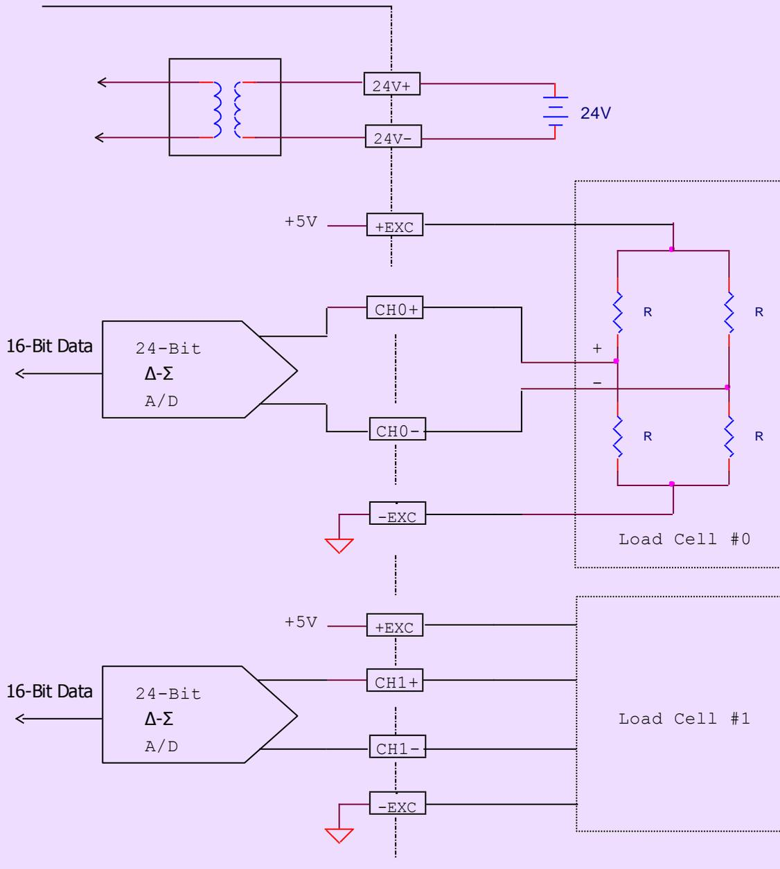
The raw conversion result is represented by a 16-bit signed value. After setting the full range engineering value and perform the zero and full scale calibration procedure, the system will automatically convert the raw conversion reading value into engineering weight value for user application.
