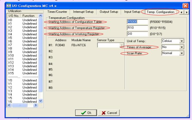
The user needs to assign a starting register of a contiguous register area for Configuration Table,
