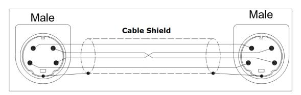
b. Wiring diagram of cable for PEP and P1/P2/P3/P4 RS232 connection
