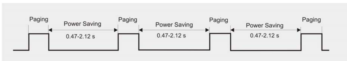
Figure 9: Power saving and paging in GSM networks
