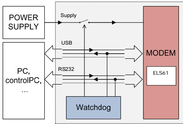
Time, which is still not considered an error of modem is configured using commands via serial interface RS232. USB port is not possible to use for Watchdog setting!
