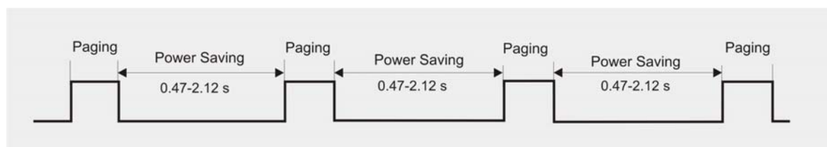
Figure 34: Power saving and paging in GSM networks
