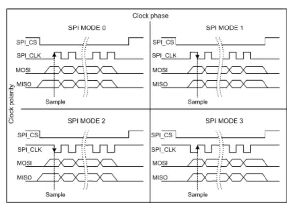
Figure 19.1: SPI modes selectable on SPI
